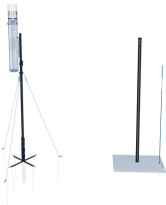
Complete precipitation observation setup.
