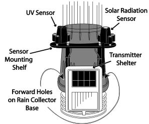
It should be noted that proper installation is still important for highly accurate readings. The ISS needs to be installed in a location that is free of shadowing by trees, buildings or other objects. Address these issues first before addressing the issues with bird spike installation.
